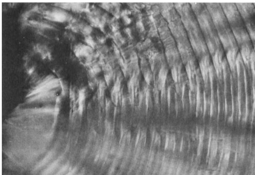
FIGURE 17 Enlarged area from picture 16, showing the double spatial periodicity associated with the half pitch Z/2 of the helix.
